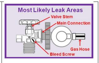
2. Check that the O-ring or rubber hood are attached to the end of the brass fitting on the regulator and are in good condition.
